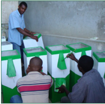
The floods contaminated many drinking sources. The ZL team recently constructed 100 biosand filters from local materials to purify water for families affected by the storms.
